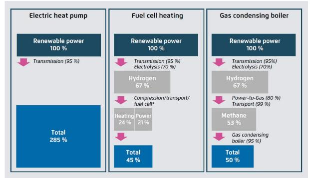
\* Efficiencies: 80% (compression/transport) and 85% (total fuel cells; 45% heating, 40% power)
